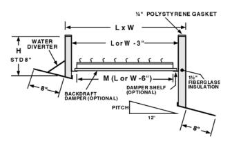
Damper shelf supported from top ledge of curb, but supported from base of curb when total rise over length > 2".
