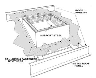
Metal Roof Curb Self-Flashing Type MRSF
